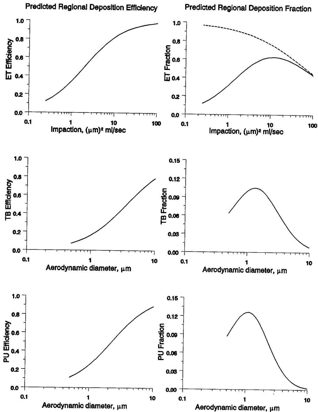
**Figure G-1. Comparison of regional deposition efficiencies and fractions for the mouse. A default body weight of 0.0261 kg (from Table 4-4) was used in these calculations. The fractional deposition (solid line) and inhalability (dashed line) are shown in the upper right panel.**
