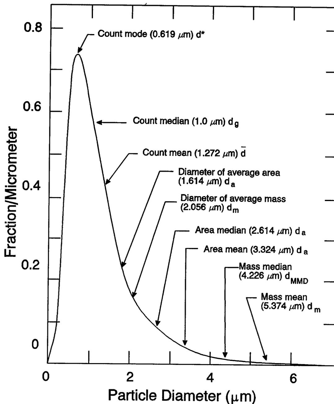
**Figure H-1.** An example of the log-normal distribution function of an aerosol. Definitions of diameters commonly used are provided in Table H-1. Note that if aerodynamic diameters were being measured, then count or other frequency distribution would be measured against that (e.g., count median aerodynamic diameter [CMAD]).
