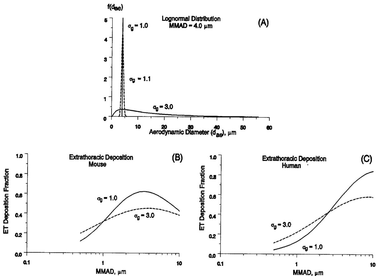
**Figure G-2.** Range of particles for lognormal distributions with same MMAD but differing geometric standard deviations (A). Effect of polydisperse particles on predicted extrathoracic deposition fractions in mice (B) and humans (C).
