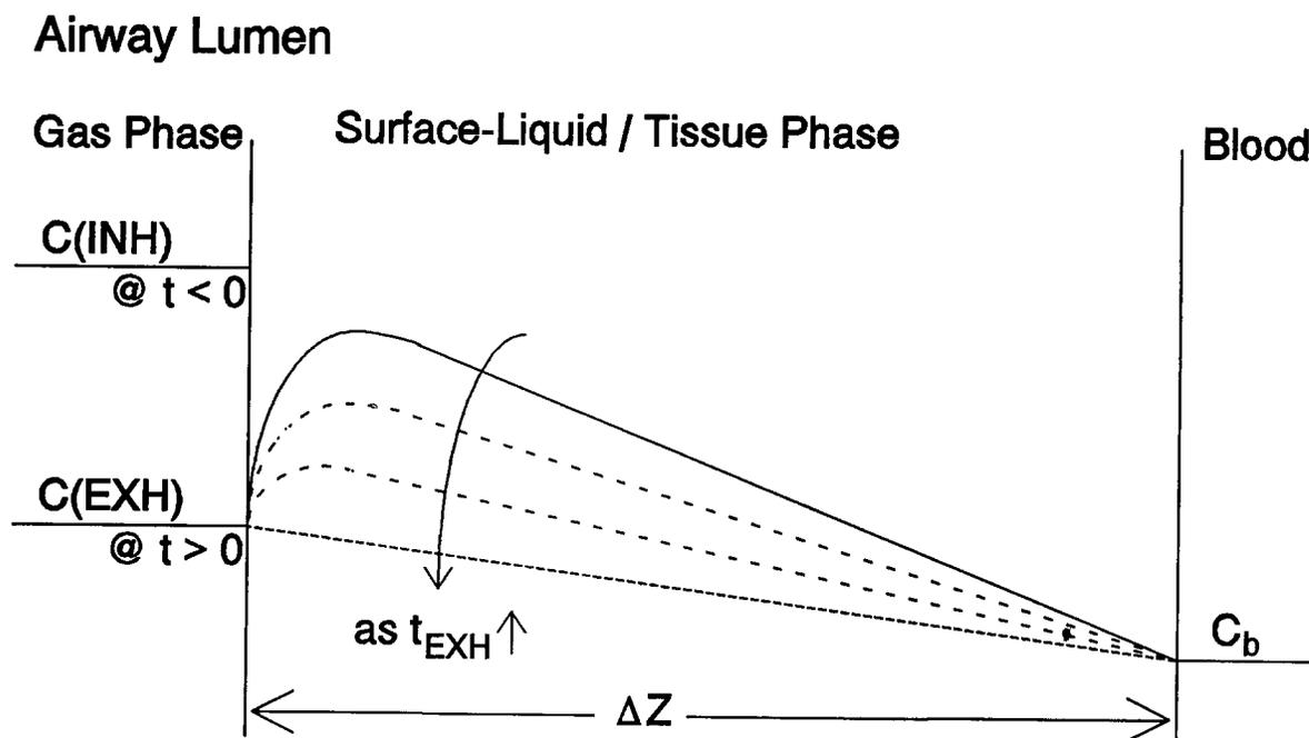
**Figure I-6. Schematic of surface-liquid/tissue phase concentration during exhalation.**
