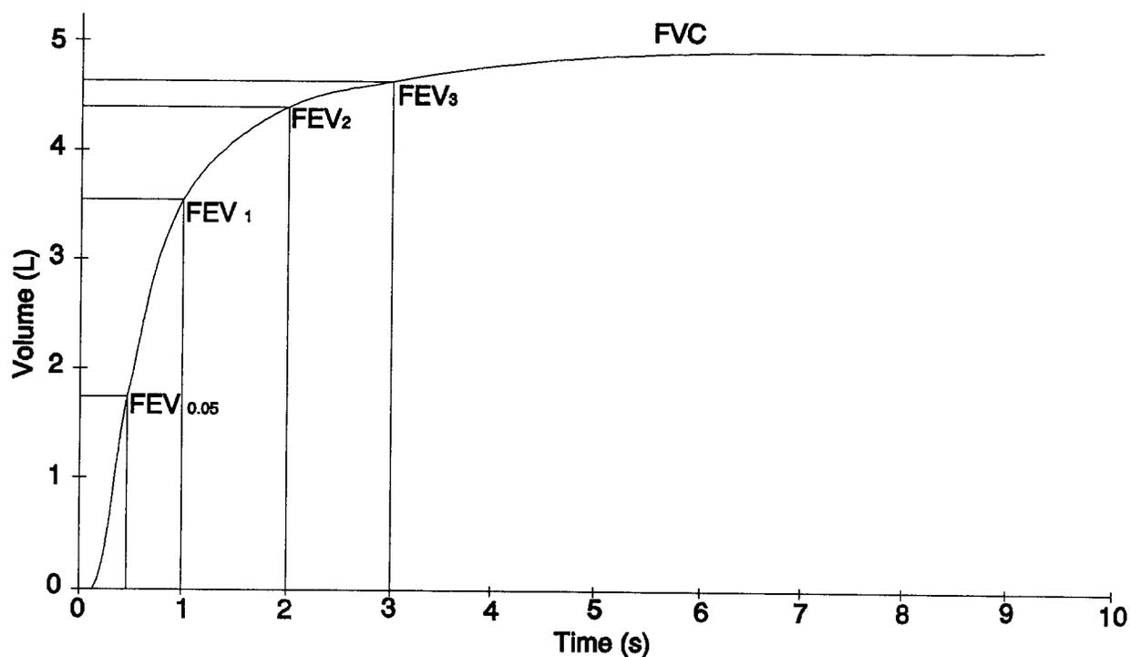
**Figure E-2.** Volume-time plot (spirogram) of the forced vital capacity (FVC) maneuver. The subject exhaled as forcefully and rapidly as possible from maximal inspiratory level. Forced expiratory volume (FEV) as various time intervals are indicated.
